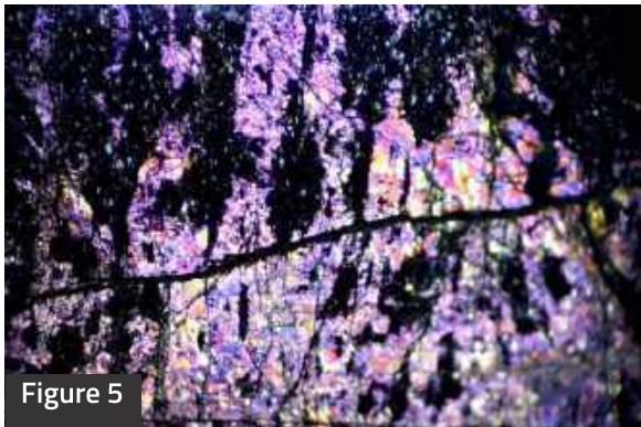
Figure 5 Fine layered structure, responsible for strong sheen and iridescence in Heterosite-Purpurite specimen. Black intermittent areas are mineral grains (also Heterosite).
