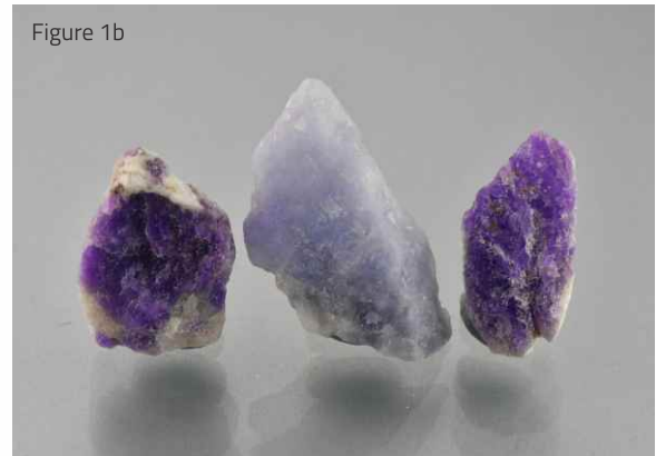
Figure 1. Rough samples of Hackmanite after fading (left) and after exposure to UV light (right). Note the intensification of purple-violet component. The sample in middle is least affected by the UV exposure but still displays some degree of colour change.
