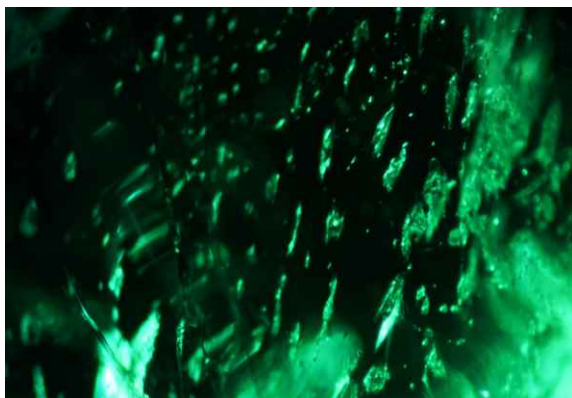
Figure 4. Whitish frosted films around 2-phase inclusions are often seen in emeralds originating from Brazil, Ethiopia and Zambia.
