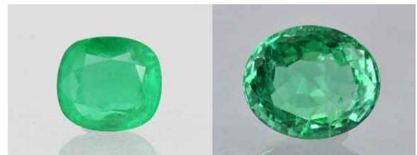
Figure 1. Faceted samples of emeralds from Brazil (left) and Ethiopia (right) displaying similar hues but reduced transparency, due to presence of minute inclusions.
