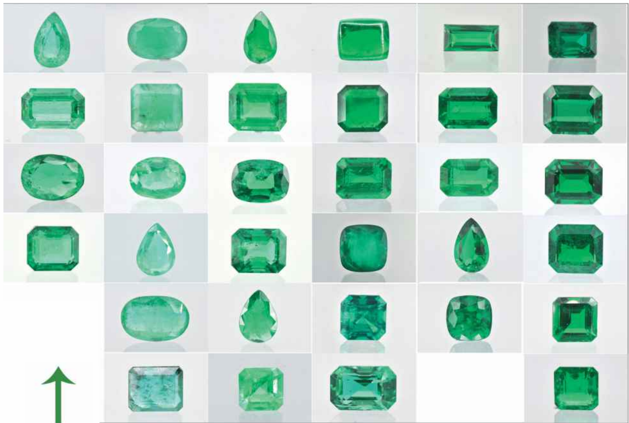
Figure 1: Chart showing colour range of emeralds from rich green to yellowish green to bluish green, in varying saturations from high (extreme right column) to low (left columns). First three columns on the left represent lighter shades of green, qualifying them for detailed analyses of their spectral features. Based on the spectral analyses, stones outlined in green are qualified as beryl and not emerald.
