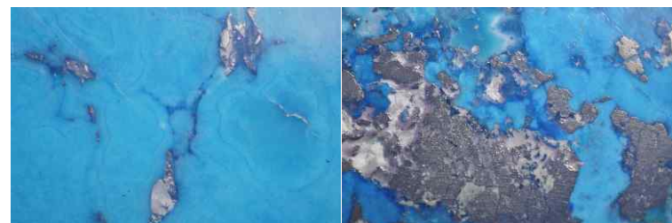
6. Filled veins and cavities in a Turquoise impregnated with coloured polymer. Note deep blue colour concentrations.
