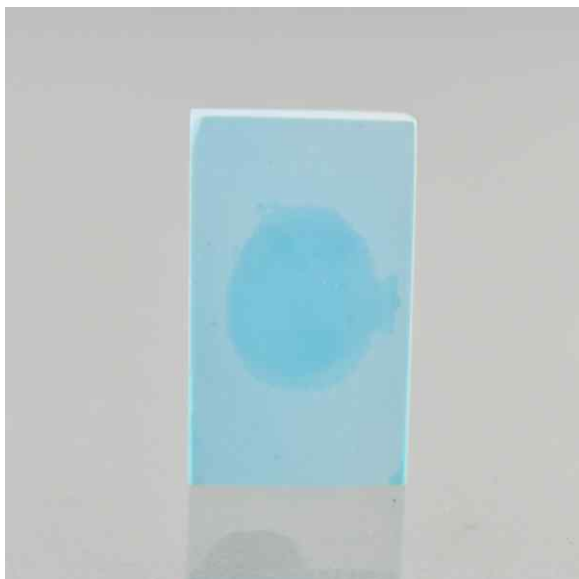
4. An illustration of effect of filler on turquoise. The image displays deeper colour on a spot applied with baby oil, while rest of the area appear much lighter.
