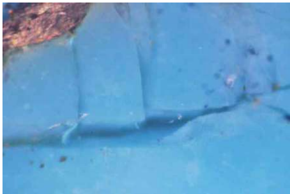
Angular fragments of Turquoise and vein of colourless polymer in a composite Turquoise.
