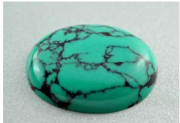
Ceramic-imitation Turquoise with and without veins (matrix). Such materials are created using grains or powder of Turquoise, Gibbsite or Barite.
