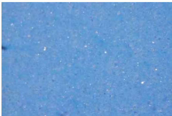
Fine granular texture in a ceramic-imitation Turquoise. This texture is typically absent in a natural Turquoise.
