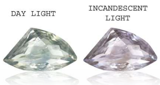
Figure 3. An example of alexandrite with weak to moderate colour change from greyish green in daylight to greyish purple in incandescent light.
