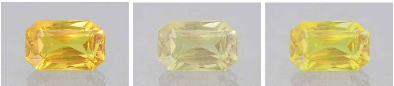
Figure 1: As received, yellow sapphire displaying a saturated yellow colour (left) fades on exposure to strong light (centre) displaying lighter yellow. Yellow colour is restored to deeper yellow on exposure to UV light (right). This suggests presence of both, unstable and stable colour centres.
