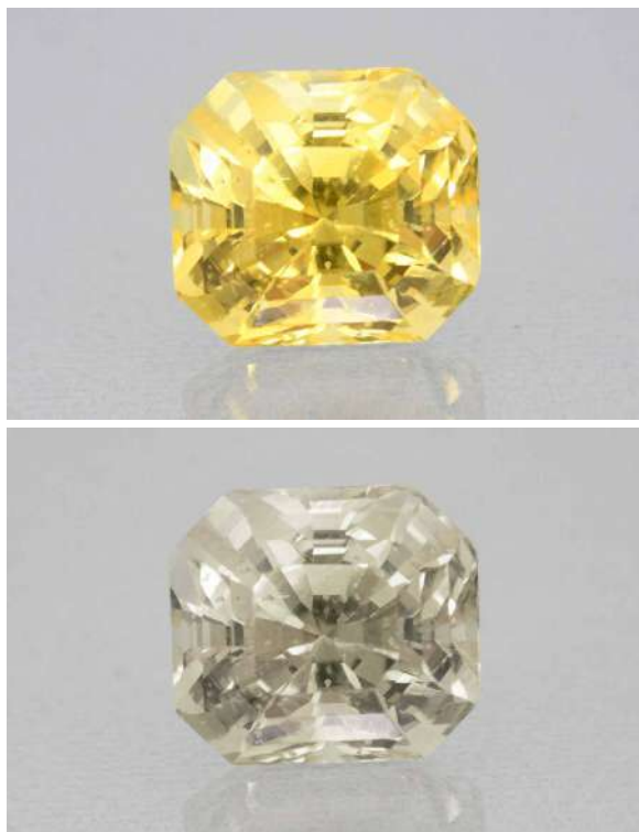
Figure 2: This rich yellow sapphire (up) fades to near colourless (down) on exposure to strong light source. This suggests presence of only unstable colour centre.
