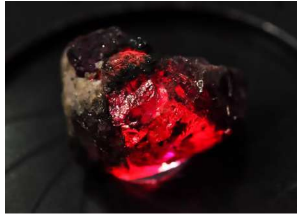
2. This bright purplish red - pink rough (top) is a composite made up of synthetic and natural ruby. The central part is a synthetic ruby while the outer part is composed of chips of natural ruby. Note the small areas of angular milky zones. Under transmitted light (bottom), central synthetic part of the specimen appeared bright red, while the edges appeared dark and opaque.
