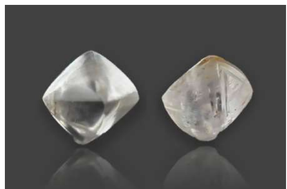
5.a. These colourless octahedrons, representing diamond, are fashioned cubic zirconia (left) and topaz (right). Also note artificially drawn triangular growth markings on octahedral faces, along with iron-stained films in topaz crystal.
