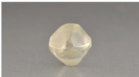
5 b. This pale yellow cubo-octahedron, representing diamond, is a fashioned synthetic moissanite, with etched surface.
