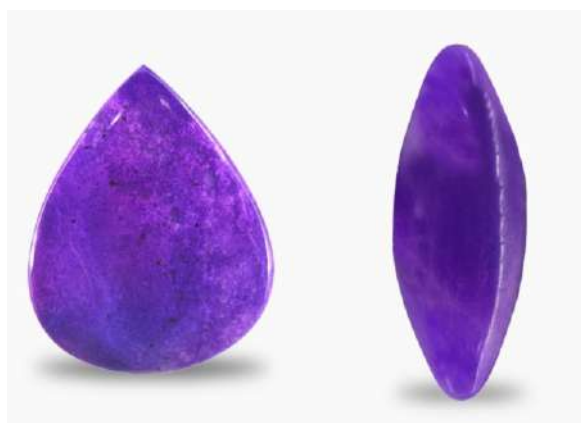
▼ Representative polished samples of dyed serpentine rock (left) and sugilite (right). Note the similarities in colour appearance and texture.
