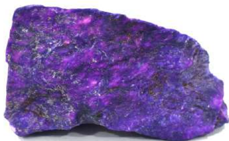
▼ Rough sample of dyed serpentine rock presented as sugilite. Note the uneven colouration
