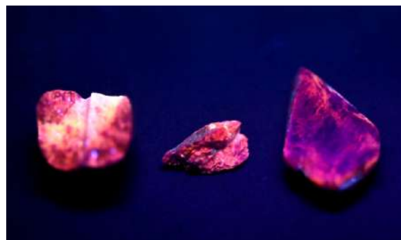
▼ Presence of artificial dye in these serpentine rock samples was characterised by strong patchy orange fluorescence in shortwave UV.
